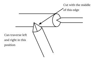
A planing cut is started with the handle well down and to the right whilst an edge is tilted to the right so that its mid point is in contact with the work. Keep the tool slanted as shown and the handle well down. The cutting is all done with the right edge. The left edge is raised a little off the work, but there is nothing to catch or dig in as the tool is rounded. The point is clear off the work and there is not back end to catch at all.
