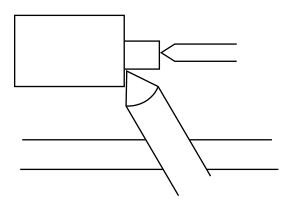
Use a top face almost horizontal, but tilted slightly to the left hand edge at 90 degrees to the lathe axis and then push towards the centre whilst gradually lifting the handle ideal for cutting shoulders or dressing the flat tops and bottoms of boxes.
