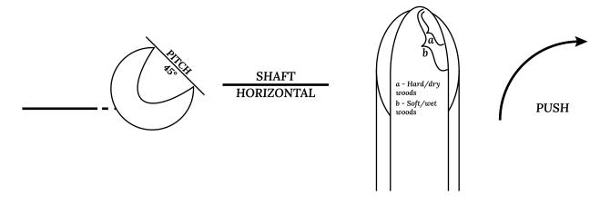
Finishing Cut: Final cut on interior surface in preparation for sanding.
